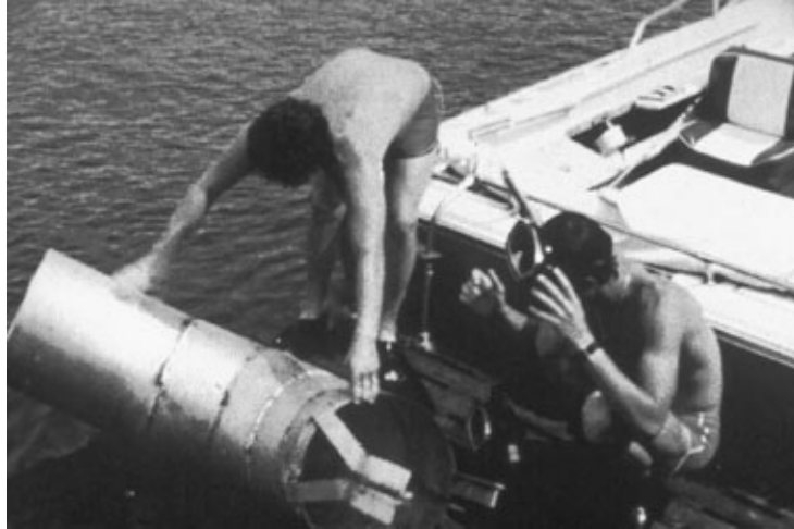
Fig. 2.2. Mike Lopez and Kenny Huertas fastening a “mailbox” sand duster to the propeller mount on our boat. We dusted the sand off the entire marble building in only a quick fifteen minutes. The propeller blast came out the bottom of the tube with truly awesome force.
